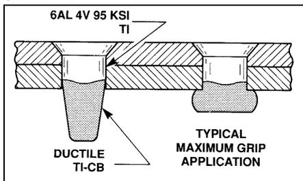
**CherryBucks** - are a one piece titanium alloy fastener. Since the fastener is composed of only one piece it is ideal for installation in FOD sensitive areas (GTE intakes). See figure 48 for a typical CherryBuck installation.
