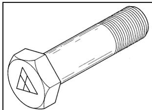
**Close-tolerance Bolts** are used where a bolt is subjected to a pounding type stress or where the final structure is comprised of both riveted and bolted members. The An173 to An186 Close-tolerance Bolts are shown in figure 55.
