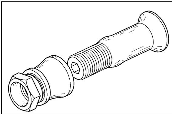
**Taper-Loks and Hi-Tigue bolts** - are the strongest form of special fasteners. The Taper-Lok has a slight taper and is installed in a conical type hole. As the washernut is tightened the fastener expands and presses into the sides of the conical shaped hole thereby locking itself into place. The Hi-Tigue bolts is tapered and incorporates a ball shaped bump on its shank, see figure 49.
