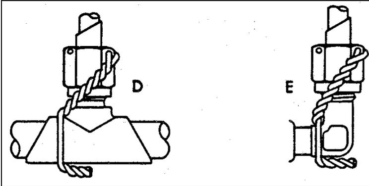
This example illustrates the correct manner to lock wire fittings when no lug or "L" bracket has been provided. Notice that the direction of wrap will pull the fitting tighter. All cut ends have been bent over.
