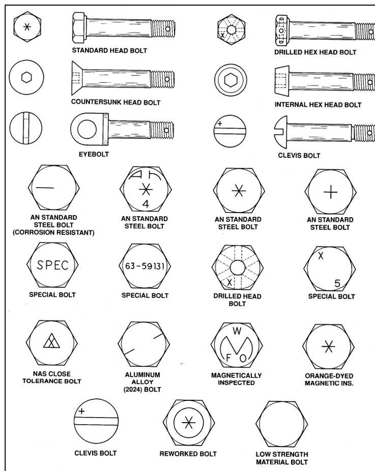
Figure 52 Typical Bolt Head Markings
