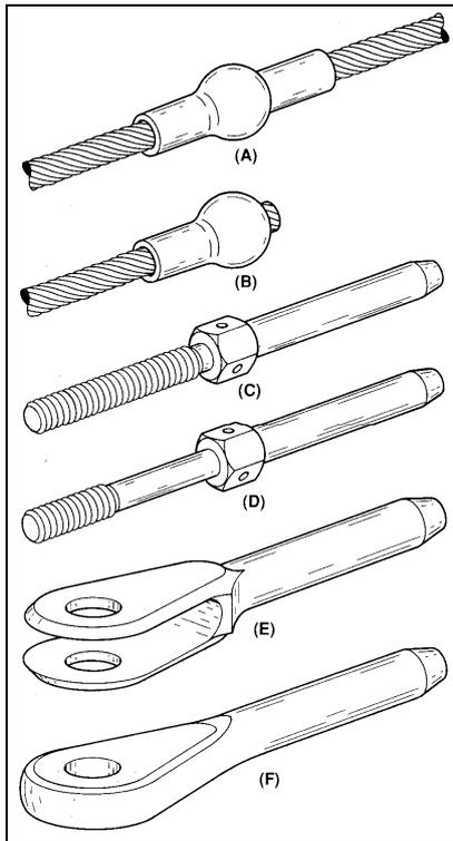
**Swaged terminals** are crimped onto the wire end using a special tool. See figure 79. Once crimped the terminal and cable is checked with a go no go gauge to ensure that the joint has been properly crimped or swaged. see figure 80.
