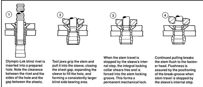
**Olympic-loks** - are a light weight,, mechanical locking, spindle type, blind rivet. These rivets are available in universal, 100° flush and 100° flush shear head styles as well as various sizes and materials. Olympic-loks are the most inexpensive self-plugging mechanical-lock rivets.
