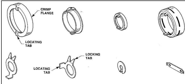
**Tab Washers** are washers that have been produced with a protruding tab(s). In use, the tab will fit into a recess machined into the surface of the component. In some cases, once installed, the tap is bent or crimped to prevent loosening. See figure 93 for sample tab washers.
