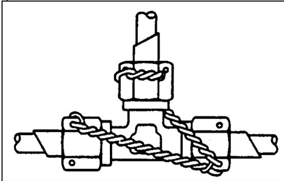
Fittings that are made of very soft materials may be lock wired as shown to prevent the wire from tearing out. Again all cut ends are bent over.
