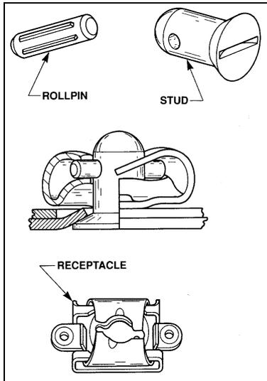
**Airlock Fasteners** consist of a steel stud and spring located on the removable piece and a spring steel receptacle on the airframe. The fastener is locked or unlocked by rotating it a quarter of a turn causing the pin to drop into an indent in the receptacle spring. See figure 75.
