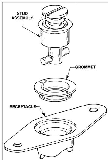
**Camlock Fasteners** use a stud and a steel pin mounted to the removable part with a metal grommet. The stud fits into a pressed steel receptacle and is locked or removed with a quarter turn. See figure 76.
