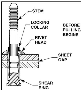
**CherryLOCKS®** - are a type of mechanical lock rivet that may be used as an in lieu replacement, with no diameter increase, for solid shank rivets. Due to the complex tools required for installation their use is usually restricted to depot and factory maintenance facilities. CherryLOCKS® are available with both universal and 100° countersunk heads and in several sizes and combinations of alloys. See figure 41 for a CherryLOCKS® rivet.
