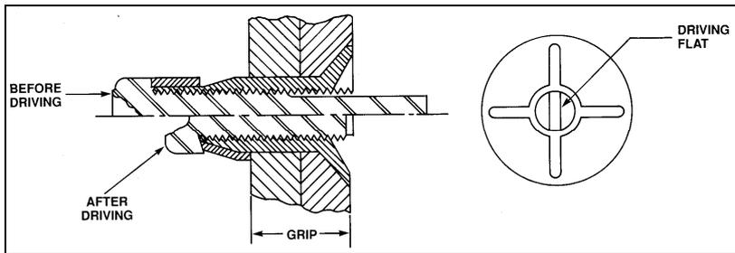
**Jo-Bolts** - are high strength structural fasteners commonly used where sufficient clearance is not available for An, MS or NAS nuts and bolts. To install a Jo-Bolt the
