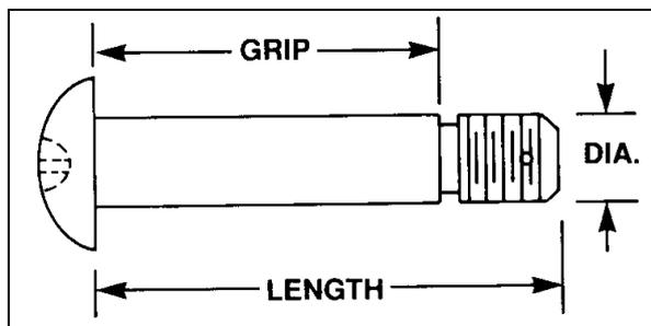
**Clevis Bolts** - are used when the assembly will encounter shear stress, only. They are commonly used to attach control cables to control horns. The smooth portion of the shank will allow the bolt to pivot while the threaded portion prevents the bolt from falling out. Both self-locking and cotter pin type nuts may be used with a Clevis bolt. See figure 56 for an example of a Clevis bolt.
