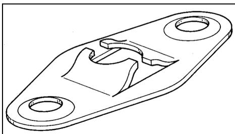
Figure 62 Anchor Type Tinnerman Nut
