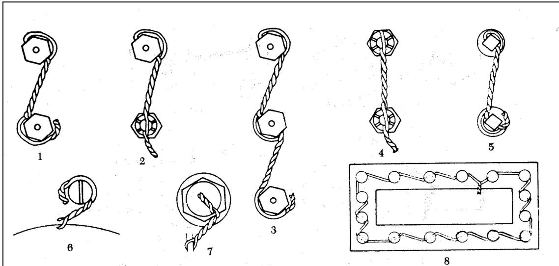
In each example the wire has been run through a hole in the fastener and then twisted around the fastener head so as to pull it tight. The twisted wire is then run to a fixed point. One fastener may be run to another but care must be taken to ensure that each fastener is preventing each other from loosening. In all cases the specific manufacturers instructions should be followed.
