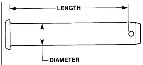
Figure 68 Aircraft Clevis Pin
