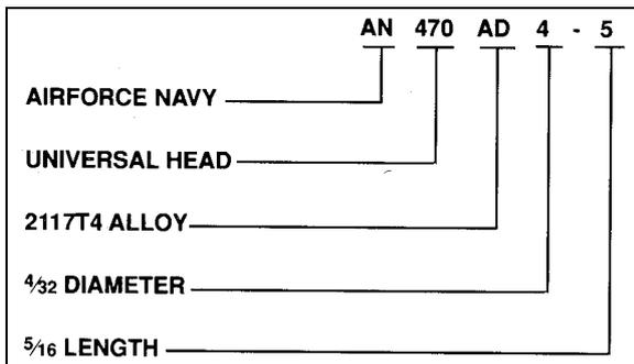
**Figure 36 Rivet Identification**
