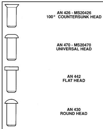
*The countersunk heads will allow the rivet to be flush mounted to increase aerodynamic efficiency and to lessen drag. The surrounding metal may have to be countersunk or dimpled in order to install countersunk head rivets.*
