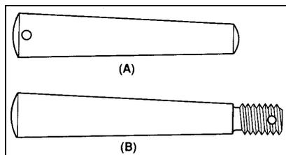
Figure 70 Aircraft Taper Pin
