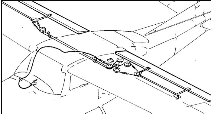
Figure 77 Steel cables are used in many aircraft to perform control functions. Cable is light, strong and its flexibility allows it to be routed through the complex airframe. One disadvantage however is that changes in temperature will cause the cable to lose tension and change the control "feel". In larger aircraft an automatic tensioning system is often used while in smaller aircraft the cables are adjusted to a compromise
