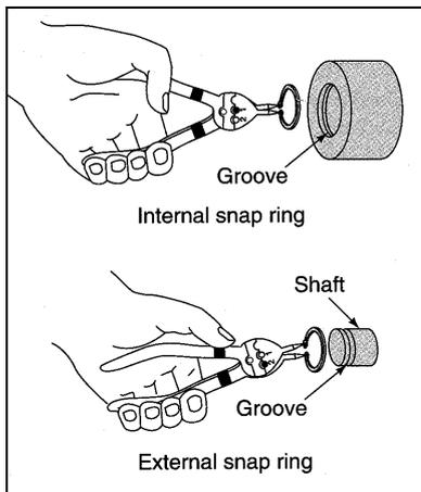
Figure 90 Snap Ring Install/Remove
