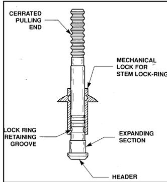
**Huck-Loks** are a type of mechanical lock rivet that may be used as an in lieu replacement, with no diameter increase, for solid shank rivets. Due to the complex tools required for installation their use is usually restricted to depot and factory maintenance facilities. Huck-Loks are available in several sizes and combinations of alloys. See figure 40 for a typical Huck-Lok rivet.
