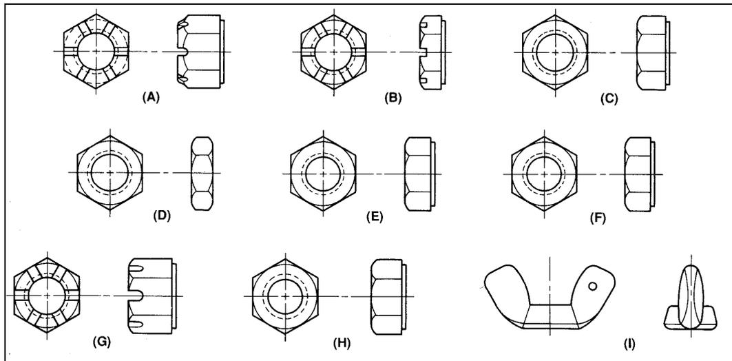
Figure 58 Non Self-locking Nuts
