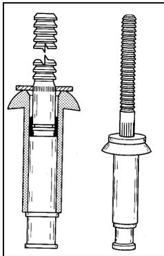
**CherryMAX®** - rivets are both economical and strong. Only a single sized installation tool is required to install all sizes of CherryMAX® rivets. The rivet is available in both universal and countersunk head styles and in various alloy compositions. See figure 43 for a typical Cherry MAX® rivet.
