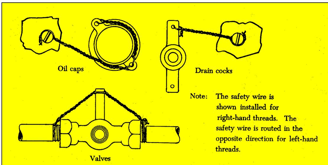
As in the first example the wire is fed through a predrilled hole, twisted and then run in such a manner so as to prevent the part from loosening.
