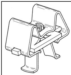
The **Tinnerman Instrument Mounting Nut** consists of a nonmagnetic, phosphor bronze cage containing a brass nut. The Tinnerman nut is used to mount instruments and controls in an instrument panel. See figure 61 for an example.
