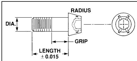
**Internal Wrenching Bolts** - are used primarily for tensile loads. They are installed using an Allen Wrench and they require a countersunk hole. See figure 57 for a typical Internal Wrenching Bolt.
