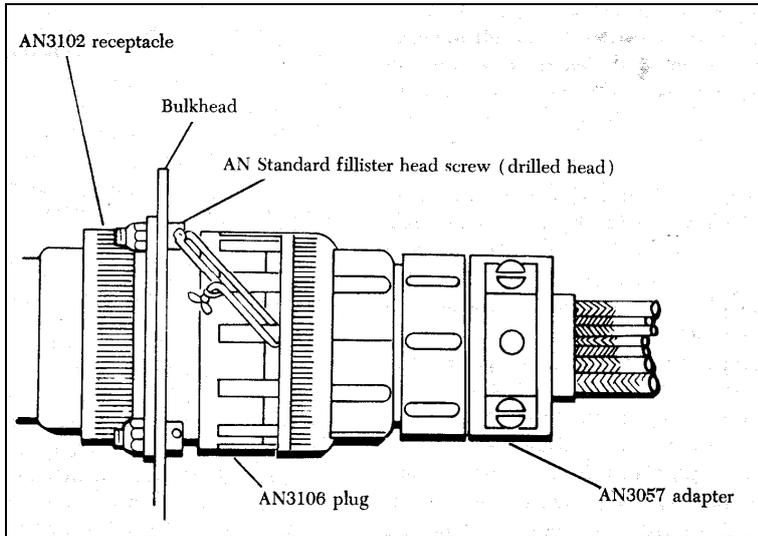
In this example the wire has been run through a predrilled hole on the collar of the plug, twisted and then fastened to a Fillister Head screw. Care must be taken to ensure that the wire is tight and is pulling the collar clockwise. Ensure all cut ends are bent over.
