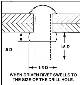
*As the rivet is driven the cross sectional area will increase. The bearing and shear strength will also increase as the metal is "worked".*
