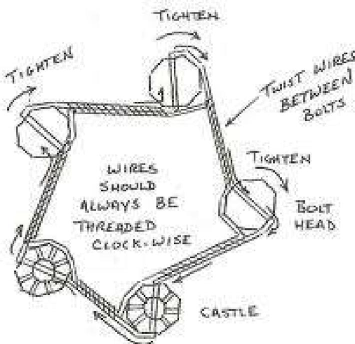
If a series of closely spaced components are to be lock wired a single strand of wire may be used if specified by the manufacturer. Any number of closely spaced components may be lock wired together however the maximum length of a single piece of lock wire shall not exceed twenty-four (24) inches.
