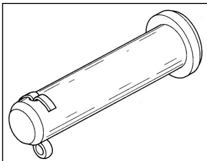
*The clevis pin may be used as a safety pin. in this case it is secured with a small cotter pin.*
