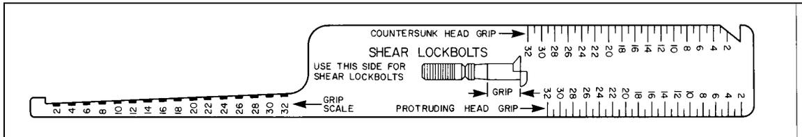
Figure 44 Lockbolt Thickness/Length Gauge
