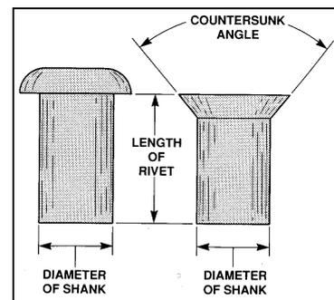
**Figure 37 Rivet Measurements**
