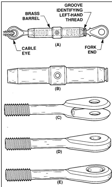
**Turnbuckles** are used to adjust cable tension. A complete turnbuckle will consist of a brass barrel, an end piece with LH threads and an end piece with RH threads. Once adjusted the turnbuckle must have both ends safety wired to prevent loosening. See figure 82.
