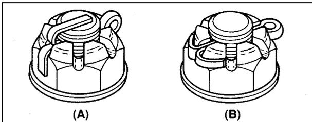
**Cotter pins** are used throughout the aircraft to prevent movable parts from separating. Cotter pins are installed through a predrilled hole, the legs are spread and then bent over to keep the pin from vibrating loose.
