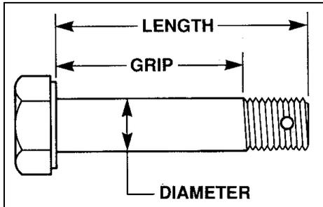
**Airframe Bolts** - are used for aircraft structural applications. The common AN3 to AN20 Airframe bolts are illustrated in figure 53. These bolts are available in cadmium plated nickel steel, corrosion resistant steel and in 2024 aluminum alloy. These bolts have National Fine Threads with a Class 3 fit.
