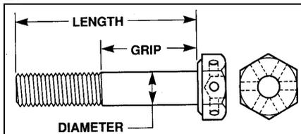
**Drilled-head Engine Bolts** - have a small hole drilled through each of the head flats to facilitate safety wiring. The common AN73 and AN81 bolts are shown in figure 54.
