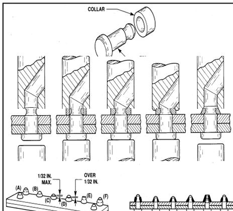
Figure 45 Hi-Shear Rivet
